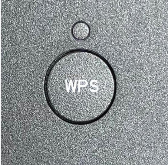
Wi-Fi Protect Setup (WPS) makes it easier to connect your Computer or other device to a secure Wi-Fi connection. If you want to use WPS simply push the WPS button on your Arris Cable Modem TG3442. (see picture above)
