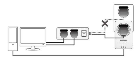
3. Please note that 200Mbps (Edimax HP-200x series) and 500Mbps (Edimax HP-500x series) powerline adapters are able to communicate directly with one another. 200Mbps and 500Mbps powerline adapters can be used on the same household electric wiring as 14Mbps & 85Mbps powerline adapters (Edimax HP-85XX series) without interfering, but are not able to communicate directly with 14Mbps and 85Mbps powerline adapters.
