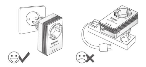
2. If you need to use a multiple socket for additional network devices, then connect the multiple socket to the integrated power socket of the adapter, and plug the powerline directly into a power socket, as shown below. The power socket of the adapter features a filter function which is able to improve the data transmission in the network.
